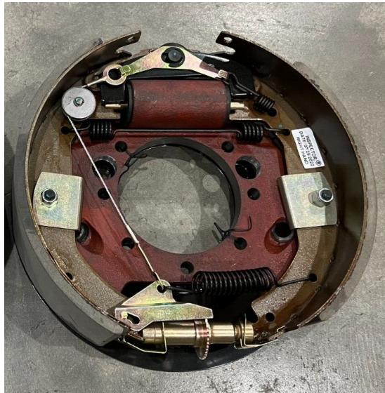
**RH 12-1/4" x 5" HYDRAULIC Brake Assembly 7 Hole Mount Fits Dexter 12K / 15K axles**
